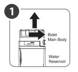
Turn and pull the bidet body out from the water reservoir.
