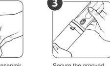
Secure the grooved end and align the notch, rotate to lock water reservoir by matching the notches.
