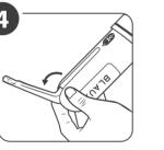
Pull the notch of the cleaning wand base to deploy.
