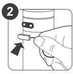
Connect the magnetic plug to the bidet to start charging. The magnetic connector can only be placed in one direction. The LED indicator near the buttons will be lit solid RED when charging.
