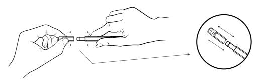
The bidet nozzle orientation can be changed depending on your handling preference. To change the nozzle, hold the nozzle firmly and pull from the wand. The nozzle is tightly fitted and require some force to undo, this is normal for water sealing purpose. Please inspect the water seal O-ring on the wand before inserting the nozzle. Orientate the nozzle (front or backward facing), push-in to fasten.
