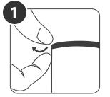
Use your fingernail to lift the color ID ring from the base of the water reservoir to remove.
